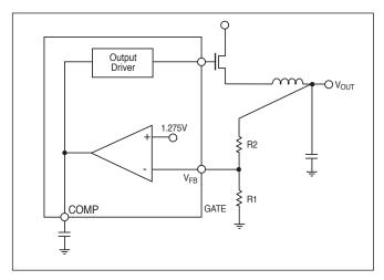
Figure 3: Feedback resistor divider.
