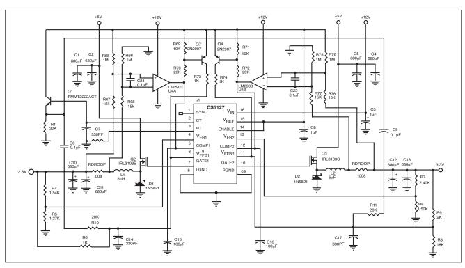
Figure 17: 200kHz,  $V^{\text{2TM}}$ , 5V/12V input, 2.8V@ 7A and 3.3V @ 7A outputs with current limit.
