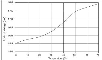
Figure 43: GATE High Voltage (100mA) vs Temperature.
