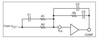
Figure 11: Two pole-two zero compensation network.
