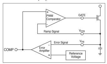
Figure 1: V<sup>2TM</sup> control diagram.
