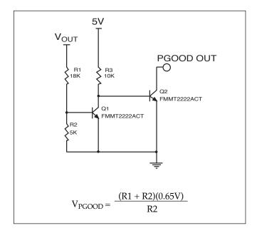
Figure 13: Example external Power GOOD circuit.  $P_{\rm GOOD(OUT)}$  is low until  $V_{\rm OUT}$  exceeds  $V_{\rm PGOOD}$ .  $V_{\rm PGOOD}$  is typically chosen to be 10% below nominal  $V_{\rm OUT}$ . Resistor values above provide a -10% tolerance on  $V_{\rm OUT}$  =3.3V.
