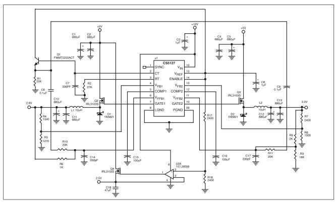
Figure 18: CS5127 12V, 5V input to 2.8V @7A and 3.3V @ 7A Switching Regulator with External 1A, 2.5V Linear Output for Vclock.
