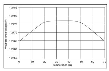
Figure 30:  $V_{FB}$  Reference Voltage vs Temperature.
