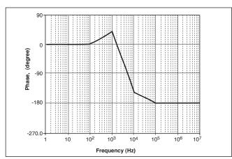
Figure 8: Bode plot of phase response for V<sub>OUT</sub>/V<sub>CONTROL</sub>.
