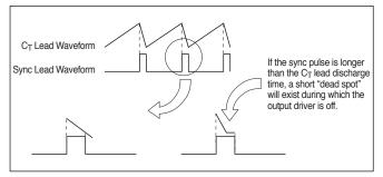
Figure 2a: Sync pulse duration vs. C<sub>T</sub> lead discharge time.
